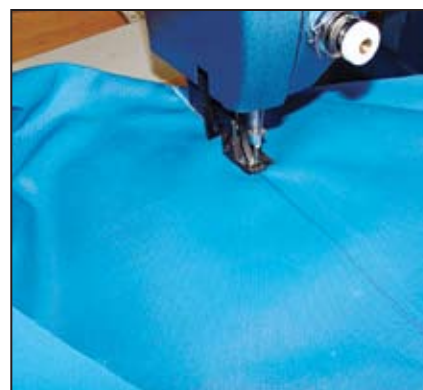
(top) Fold the seam lines over on top of one another. (bottom) Now, sew on top of the matched seam lines just inside the double-sided tape.
