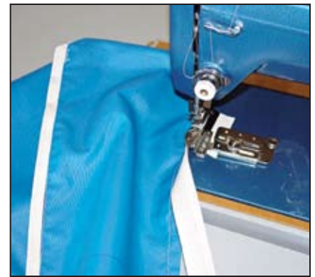
Use a binder attachment to cover the raw edges of the seam allowance to prevent unraveling.
