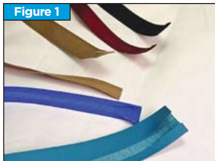
(bottom to top): Fabricated Stamoid vinyl facing; prefolded Stamoid vinyl 1" (25mm) bias binding; centerfold 7/8" woven acrylic (22mm) binding; 1" (25mm) webbing; and prefolded 3/4" and 1" (19mm and 25mm) Sunbrella acrylic binding.
