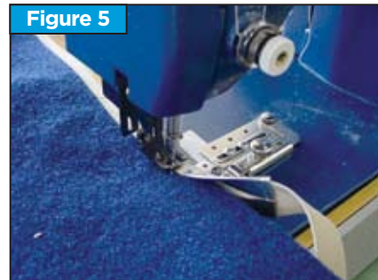
Using a swing-away binder to install 1" (25mm) binding on Boat Blanket.
