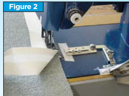
Sewing a vinyl facing good side down along the 1/2" (12mm) fold edge to Berber carpet. Notice binder in swing away (unused) configuration.
