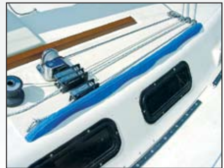
Completed cover secured to handrail with Velcro. The top stitch is a nice looking detail.
