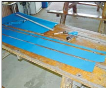
Two side rectangles and top rectangle cut for a handrail cover.
