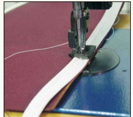
Figure 12 Sewing the welt to the right side of the first plate. By sewing in a clockwise rotation keeps the bulky material to the outside.
