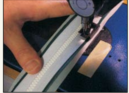
Figure 7 (top) Matching the zipper to the placket. (bottom) Sewing along the zipper teeth.
