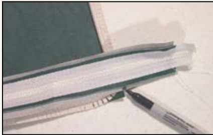
Figure 18 Mark the first corner point then each corner in succession as you sew.
