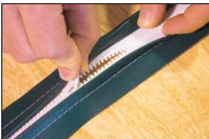
Figure 9 (top) Starting the zipper slider with the pull-tab on the right side of the placket. (bottom) While feeding the slider the zipper opens up ahead of the slider.
