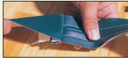
Figure 16 The seam that joins the boxing to the left end of the placket.
