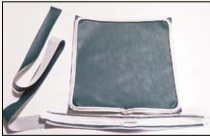
Figure 17 Lay out components in preparation to secure the placket and boxing assembly to the first seat plate.
