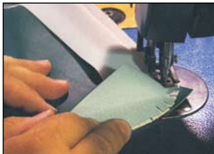
Figure 20 Notches ("eases") cut into the boxing at the corners.
