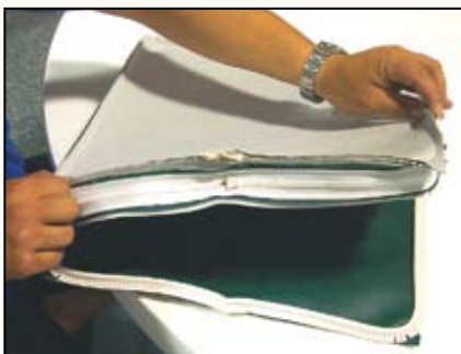
Figure 25 Matching the final plate to the boxing, placket and plate assembly. Everything is wrong side out.
