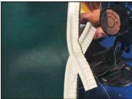
Figure 14 (top) The crossover technique to finish the welt circle. (bottom) Trimming the crossover ends.
